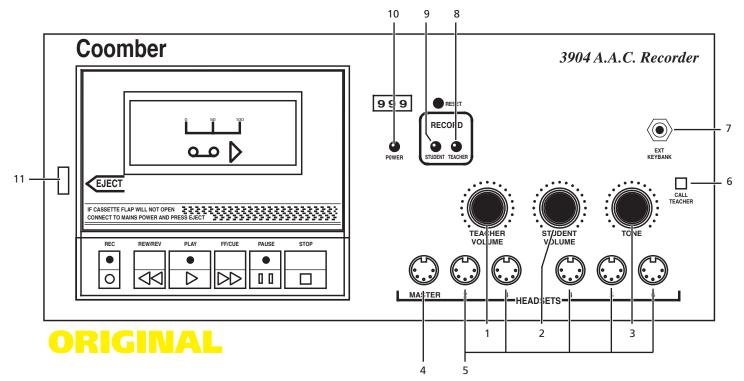
The 3904 is Audio Active Comparative. It uses the standard compact cassette, but the cassette is used on one side only. The 'Comparative' feature is obtained by using the lower half for the 'Teacher' recordings and the upper half of the 'Student response recordings.
